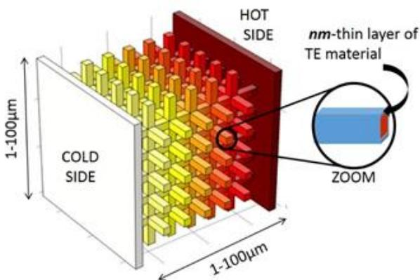
Figure 1 : 3D Thermoelectric materials obtained by two photons lithography (3DTEmat-2L). All the segments of the host polymer material are covered by a thin electroplated thermoelectric material
