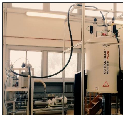
Photo of the ROMANE loop passing through an NMR spectrometer
